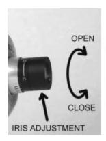
Slightly rotate the ring to adjust the iris. Avoid unscrewing the lens. The iris should be adjusted in a manner to get the maximum amount of light within the focus range without overly saturating the image.
